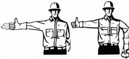
Boom up, lower load
